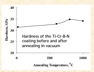
With increasing chromium content the Ti-Cr-B-N coatings showed improved adhesion strength and oxidation resistance, whereas their hardness decreased.
